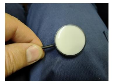
To be able to pick up under water sounds, I built me a Hydrophone to connect to my bat detector.
