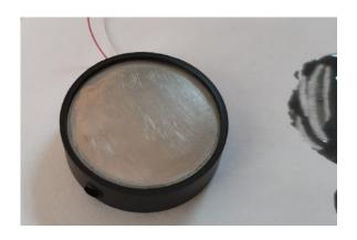
I used some epoxy glue to hold the disk in place. After the epoxy glue is set I casted the urethane on top of it being careful it does touch the edges to seal it from the water.
