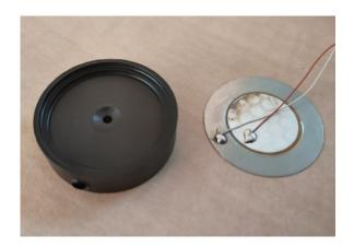
This is the end where I put the piezo disc, there is just enough space so the blobs of solder can not touch the back of the housing.
