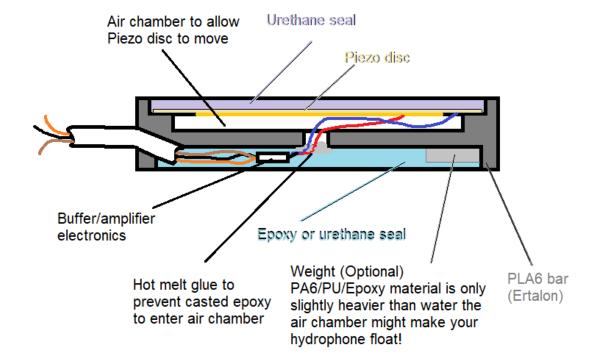
As you can see I still covered the Piezo disc with a small layer of 2-component casting urethane to have some extra protection.
