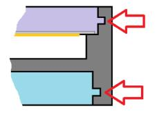
This a detailed image of the extra cut out I made Only a small cut of about 1\*1mm is made here.
