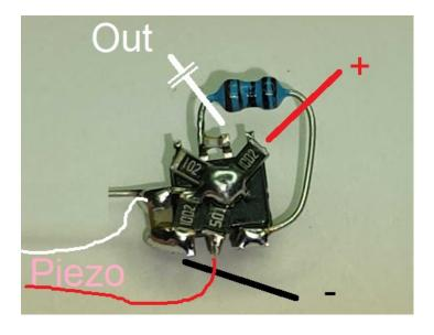
I soldeded my impedance buffer/ amplifier dead-bug style on an SMD TL972 dual operational amplifier.
