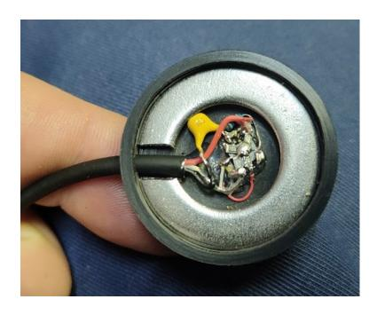
C2 is not visible in this picture. I used an M16 washer to add some weight. All though the air chamber is quit small I added the weight to be sure it will be sinking The Polyamide housing and Urethane is near the density of seawater.
